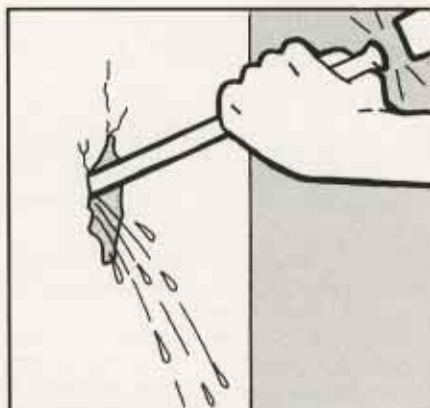
Surface preparation by chiselling
